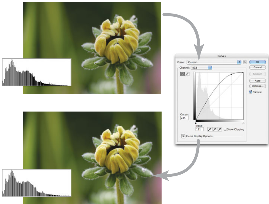
FIGURE 11.54 To restore some lost brightness, we apply another point in the highlight region of our curve. Our curve now has two additional points, and the contrast in the image is improved.
